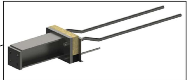
Sapphire Anchor Penetrating Exterior Insulated Steel Framed Wall with Sliding Glass Door
