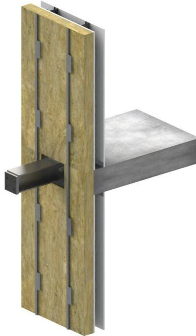
**Figure 2:** Detail 1, Sapphire G60/G25 through an exterior insulated steel framed wall
